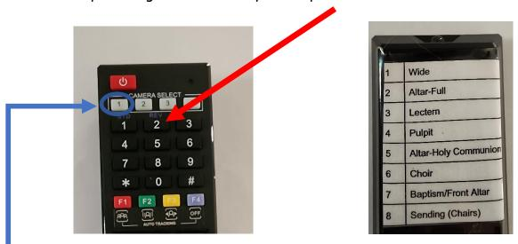
If nothing happens, press the WHITE 1 camera select button to make sure it's on camera 1 and push black number 2 button again (same button as in step 2). The camera should move.
