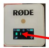
The receiver (RX) should show both the RX and the TX with full charge and you will notice the sound bar moving when there is sound.
